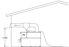
Figure 22 – Sidewall Venting
